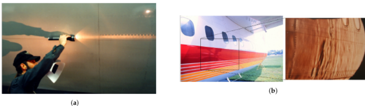
Figure 1. An example showing pillowing corrosion and surface micro deformations. (a) A specialist using a flashlight performs fuselage visual inspection; (b) the fuselage photo scanned showing surface micro perturbations caused by corrosion.
