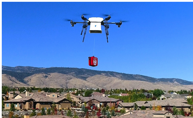
A quadcopter delivers an automated external defibrillator (AED). © 2017/Mollyrose89
