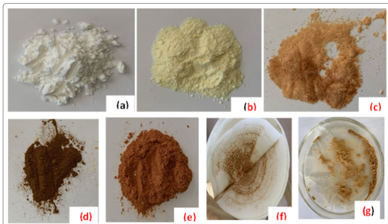
Fig. 2 Digital photographs of: a Native cellulose powder, b oxidized cellulose, c modified cellulose (DiGu.MC), d Cu(II)-DiGu-MC, e Hg(II)-DiGu-MC, f Pb(II)-DiGu-MC and g Cd(II)-DiGu-MC
