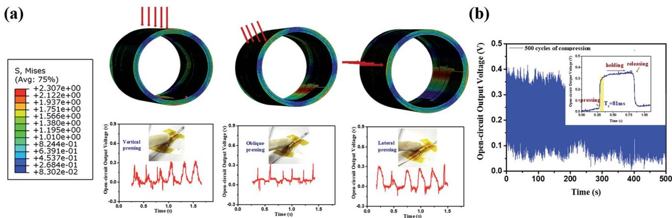
Fig. 2 Studies on piezoelectric features of TS: visualization of stress at the vertical, oblique and lateral direction with a piezoelectric output at the corresponding compression direction (a); the piezoelectric performance after 500 cycles with the inset of the piezoelectric output after one cycle (b).
