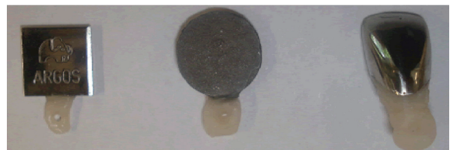
Fig. 1. Photographic representation of the different test specimens with the suspension point.
