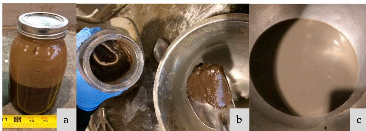
Figure 2. Ash treatment process (this process was used for SF-T, RSA-T, and RHA-T); (a) ash being soaked in NaOH; (b) ash after 24 h soaking; (c) dispersed treated ash in the activator solution.
