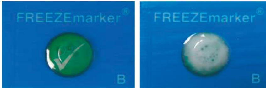
FIGURE 1. FREEZEmarker ® L visual freeze indicators maintained at temperatures higher (left) or lower (right) than their specified freeze set point. Left, Colloid is clear, allowing the green background to be easily visible. Right, Colloid has irreversibly agglomerated, preventing the green background from being visible, thereby indicating exposure to temperatures at or lower than the set point.
