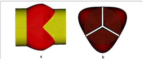
**Fig. 2** Finite element mesh of neo-aortic root. The geometries were meshed with shell elements. Three leaflets were meshed with triangular elements, and other parts of aortic root were meshed with quadrilateral element. **a** long axial view of reference model A; **b** short axial view of reference model A
