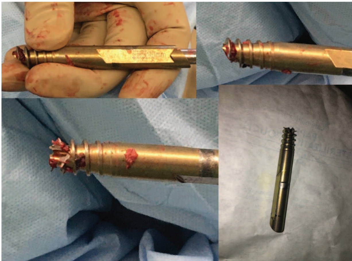
Figure 7. Intraoperative and postoperative clinical images showing explanted failed implant with breakage through the cephalic lag screw fenestrations.
