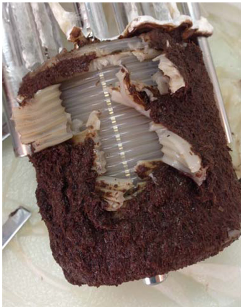
Fig. 2 Picture of an Irpex lacteus biofilm that has sequestered solid beechwood particles from the liquid phase (Brethauer et al. 2017)
