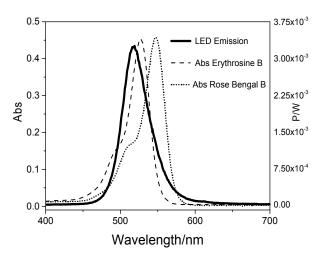
**Figure 1.** Light-emitting diode emitted potency ( $P_{LED}$  emitted) and absorbed potency ( $P_{Abs}$ ) by ERY and RB.
