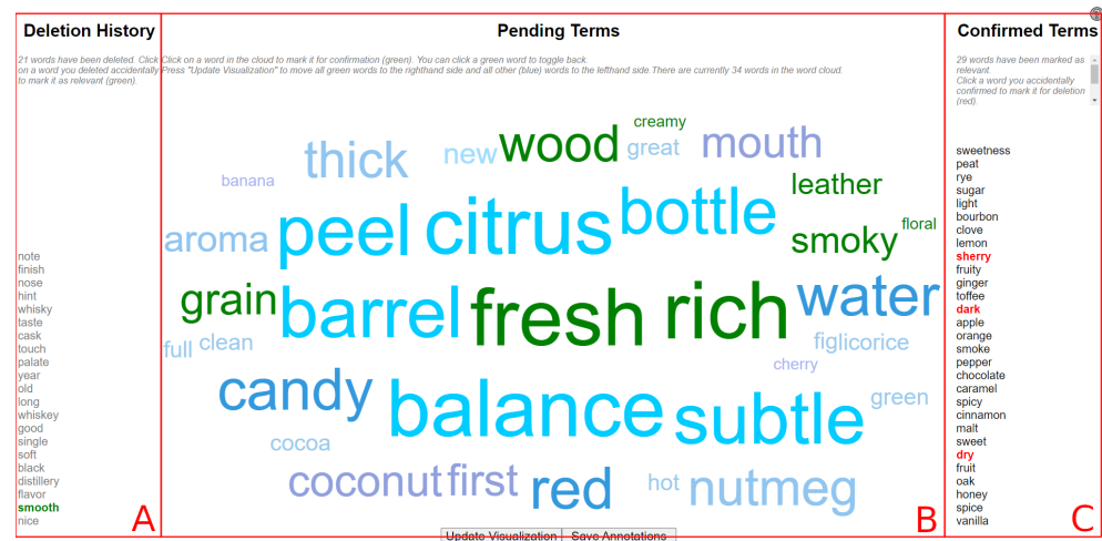
Figure 1. Interface for the Interactive Tagging Tool: (A) Non-descriptors (negative examples) are kept in the deletion history. (B) Then the most frequent words (up to 50) are shown in a word cloud format. (C) Confirmed descriptors (ones that are selected by the human operator) are stored in a confirmed terms list.
