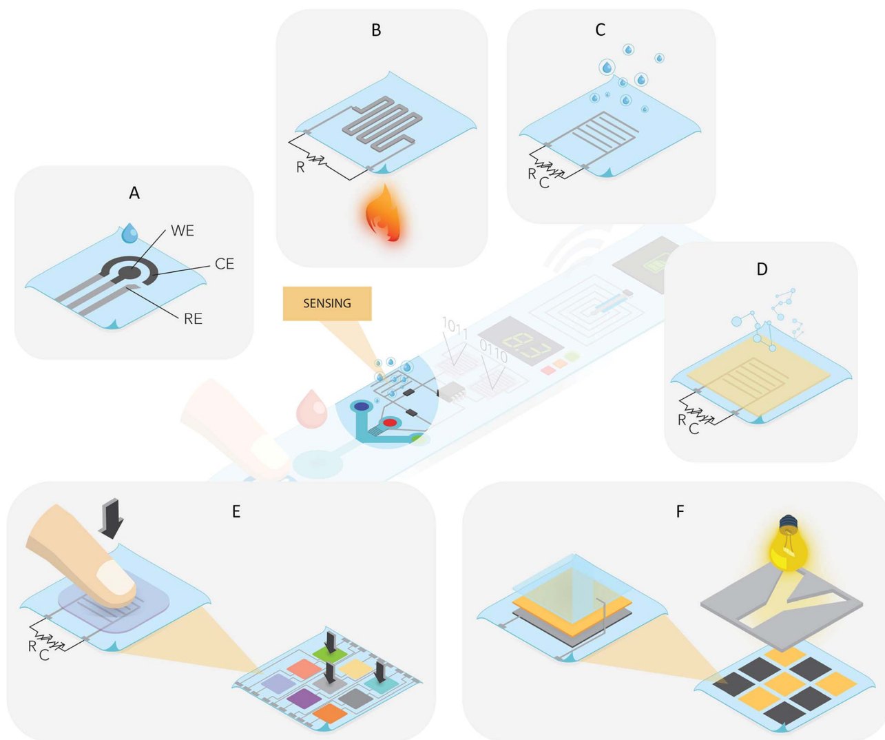
Fig. 6 Printed and paper-based sensing functional modules. (A) electrochemical sensors with working electrode (WE), counter electrode (CE) and reference electrodes (RE) indicated. Conductive materials are used for the connections and RE, while WE and CE consist of printed electrochemical functional materials. (B) Temperature sensors, with printed conductive materials and printed temperature sensitive material which varies in resistance as the temperature changes. (C) Humidity sensors, utilizing printed conductive tracks typically in an interdigitated format, which vary in resistance or capacitance as the moisture content changes. (D) Gas sensors, with a similar structure to humidity sensors but with a printed gas sensing material coating the conductive tracks. (E) Pressure, touch and proximity sensors, typically with printed pressure sensitive material over conductive tracks which varies with resistance and/or capacitance in response to pressure. These individual sensors can be implemented in matrix format to realize touch sensors. (F) Light sensors with a printed conductive electrode (bottom), printed photosensitive material (middle) and printed transparent electrode (top). These photodetector elements can also be implemented in matrix format to realize image sensors.
