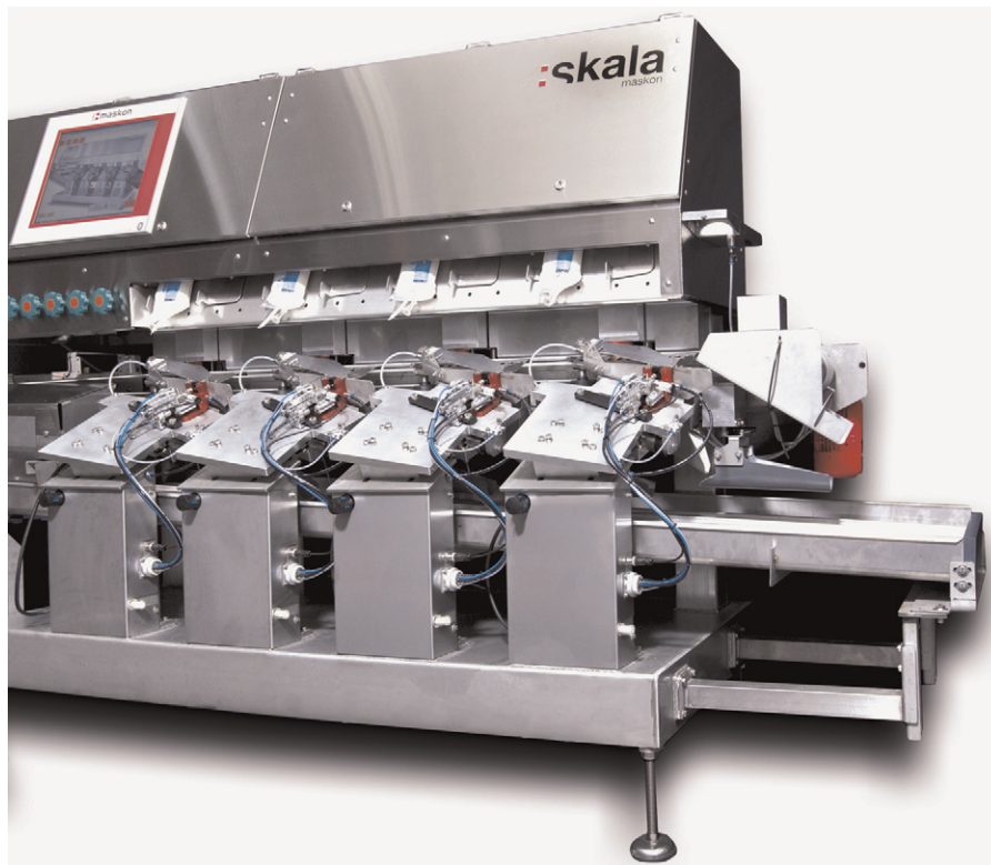
Figure 5 A vaccination system for intraperitoneal injection of salmon. Fish enter in the Maskon anesthetic and buffer tank (not shown) and are transported to the vaccination unit, which has injection sites. Location of the injection site and needle depth is adjusted for every fish based on the length of the fish. The unit is operated by one person and depending on the configuration, up to 20 000 fish can be vaccinated per hour.
