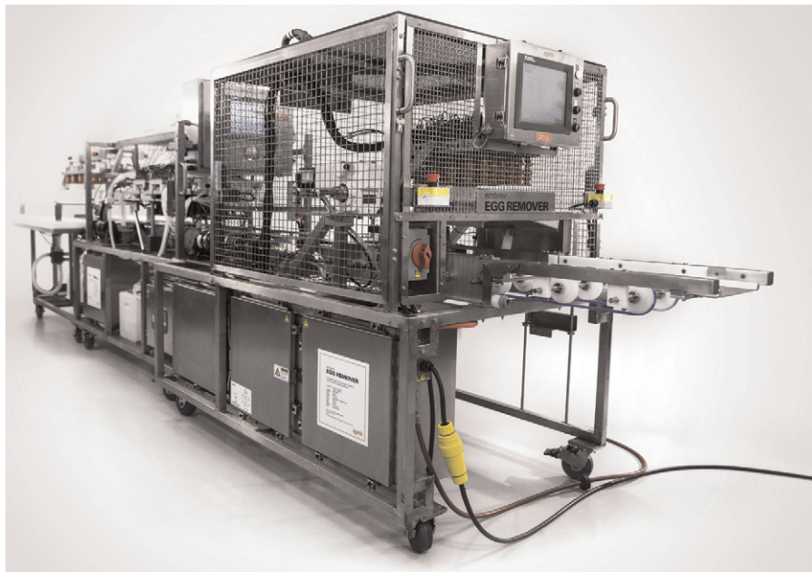
Figure 3 An automated in ovo vaccination device shown with an egg candling module and a capacity to inoculate up to 70 000 eggs h -1 . At approximately 18 days of incubation the flats with eggs are loaded on an egg remover module (right front) where infertile eggs and eggs with dead embryos are removed, thereby reducing chances of contamination. The flats are then moved to the next module for vaccine injection/delivery through a multiple-head, injector assembly that consists of a punch and needle system. After injection, the flats are moved to the transfer table module where eggs are automatically transferred to hatching baskets to be moved into the hatching incubator. Photo of the Embrex® systems (Invoject® vaccination device with Vaccine Saver® feature and egg remover module) courtesy of Zoetis Inc.
