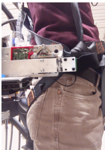
Figure 8. Human pelvis attached to the ALTACRO system from which the leg orthoses have been removed.
