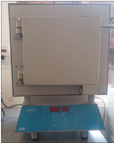
Figure 1: Photograph showing Burnout furnace
