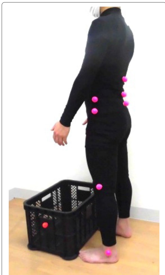
Fig. 1 The subjects were asked to lift a box (520 × 365 × 305 mm) placed on the ground. The attachment positions of the 11 markers (30-mm dia.) are shown: the subject's thoracic spine (Th12 spinous process), lumbar (L3 spinous process), pelvic (S1 spinous process), and bilaterally on the iliac crest, great trochanter, lateral femoral epicondyle, and lateral malleolus. A marker was also attached to the box
