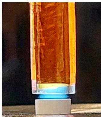
**Figure 7.** Plasma treatment on the HAP sample using the planar DBD source.
