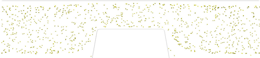
Figure 4. A side view of the cell-based PRP simulation with Q = 2.3 \times 10^{-9} \text{ m}^3 \text{ s}^{-1} in van Rooij's flow chamber at the last time step ( t = 0.35 \text{ s} ). Platelets are shown in yellow.
