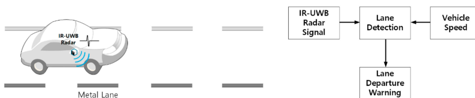
Figure 1. Metal lane detection system model using impulse radio ultra-wideband (IR-UWB) radar.
