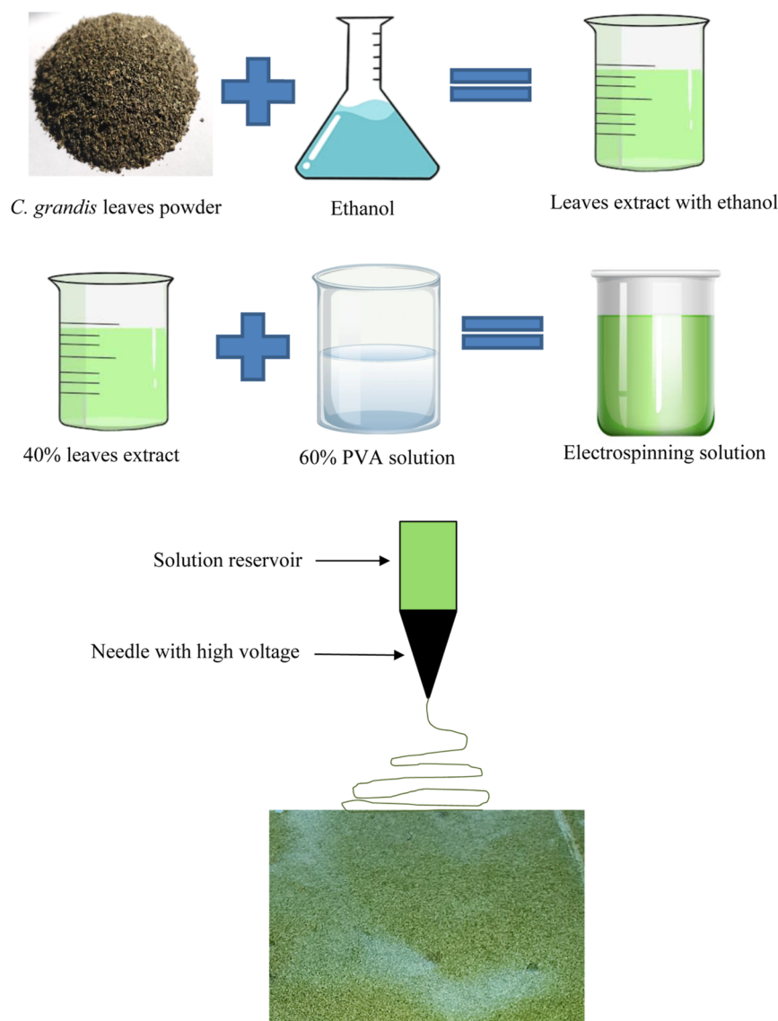
Figure 1. Schematic diagram of solution preparation and fabrication [visual representation made by Md. Redwanul Islam].
