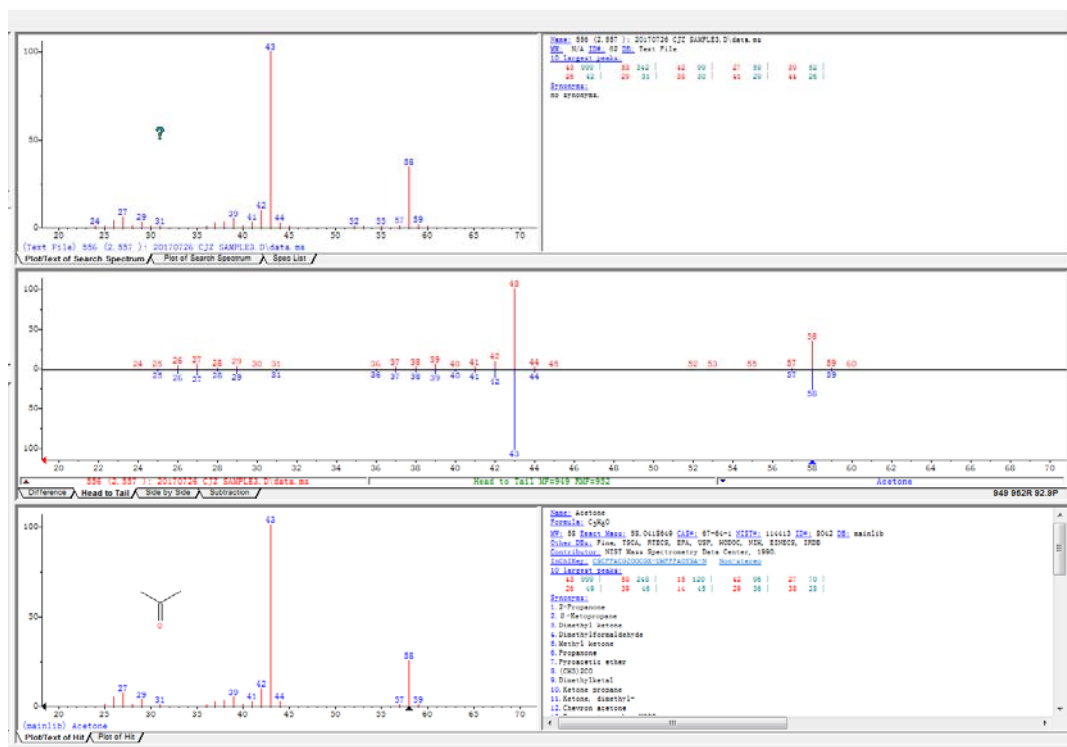
Figure S1. ESI mass-spectra of the reaction mixtures described in the Table S1: Acetone (standard sample and entry 1, peak, m/z = 43 ). Relates to the Scheme 3.
