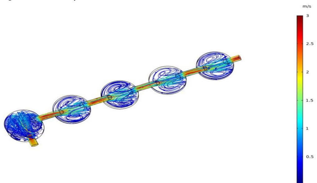
Figure 14. Simulation results of the velocity field in series cavity.
