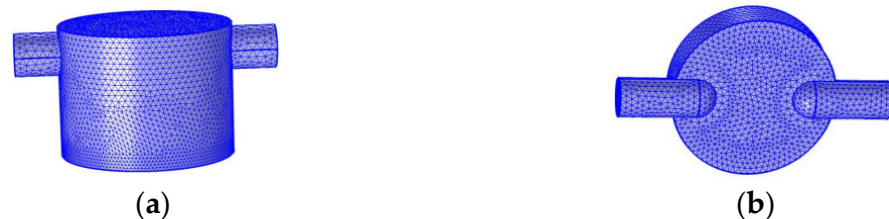
Figure 11. (a) Cover cavity airflow field gridding; (b) Cap cavity airflow field gridding.
