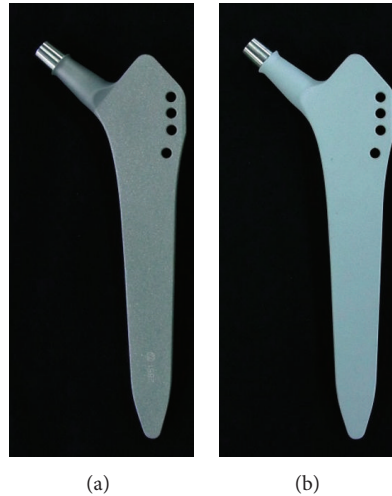
FIGURE 1: An uncoated hip prosthesis (a) and an iodine-supported hip prosthesis (b).
