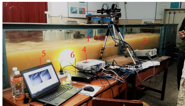
Figure 11. Experimental environment. 1. Airfoil shape; 2. binocular cameras; 3. signal generator; 4. projector; 5. laptop; 6. gigabit Ethernet switch.
