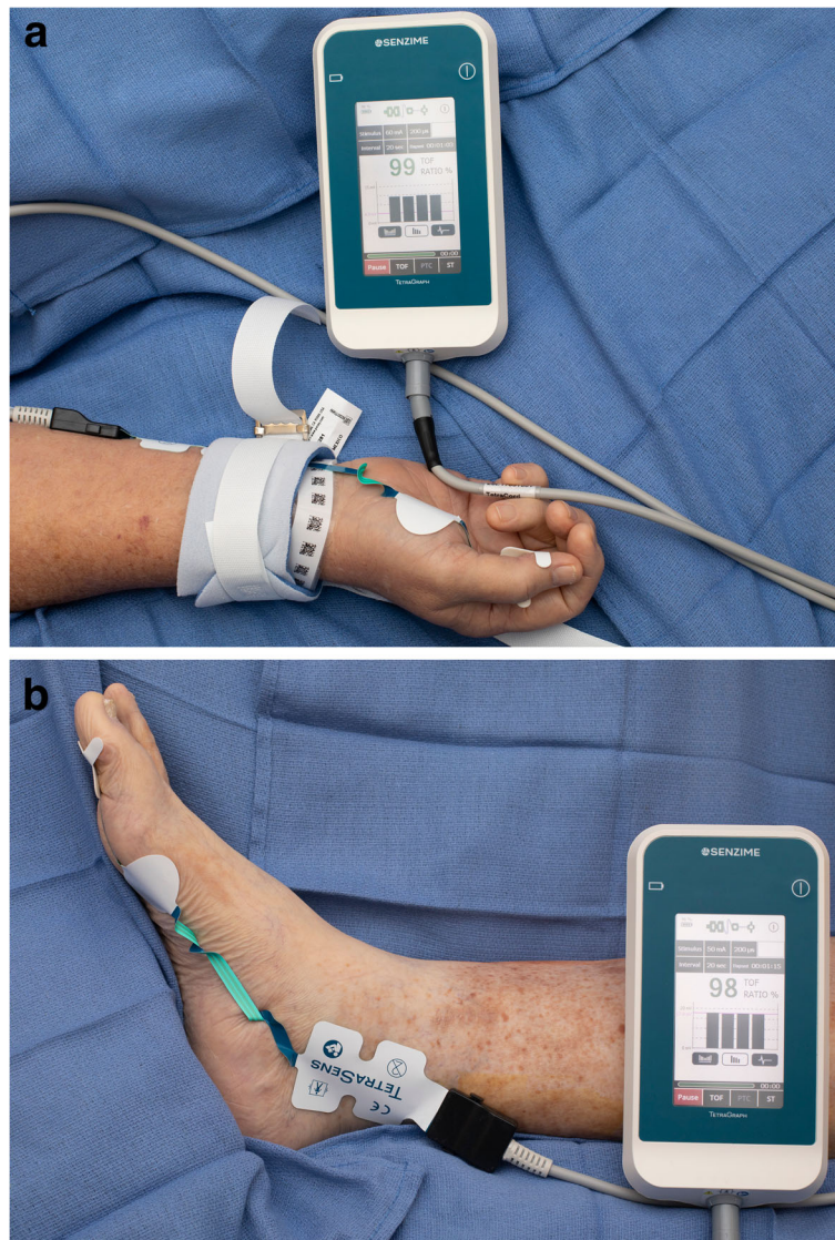
Fig. 3 a The electromyography-based TetraGraph device (Senzime AB, Uppsala, Sweden) measuring the response to neurostimulation of the adductor pollicis muscle. b The electromyography-based TetraGraph device (Senzime AB, Uppsala, Sweden) measuring the response to neurostimulation of the flexor hallucis brevis muscle
