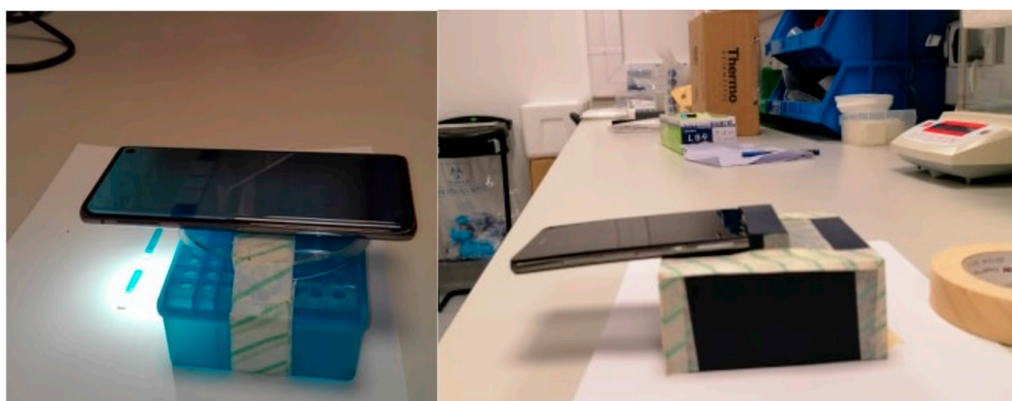
Figure 4. Left; an image of the Samsung taking an image of a LFA (the ZEU Proteon Gluten Express) under room-light conditions with the flashlight on at 5 cm distance. Right; an image of the light-shielding box used. The dimensions of the box are 11 \times 11 \times 5 cm to maintain the standard 5 cm as a distance for the photo capturing. The box had a hole in the center precisely for the camera and flash. The phone displayed on the box is the Huawei.
