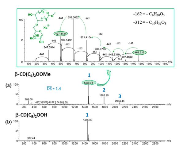
Figure 1. Electro spray ionization mass spectrometry (ESI<sup>+</sup>-MS) spectra of β-CD(C<sub>9</sub>)<sub>2</sub>OOMe 1 (a) and β-CD(C<sub>9</sub>)<sub>2</sub>OOH 8 (b). For 1 the MS/MS spectrum of the mono grafted species (m/z 1469.63) is shown. The average DS value was calculated using the following equation:  $\overline{DS} = \sum_i DS_i \times I_i / \sum_i I_i$
