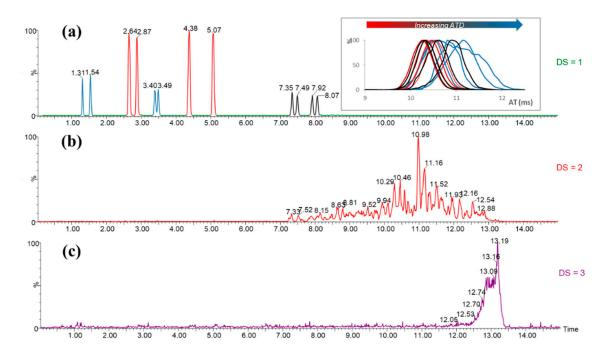
**Figure 2.** [M + Na]<sup>+</sup> extracted ion chromatograms (EICs) of **1**: DS = 1 m/z 1469.63 (**a**), DS = 2 m/z 1781.89 (**b**), and DS = 3 m/z 2094.16 (**c**). For DS = 1, the arrival time distributions (ATDs) of the 12 isomers obtained using a travelling wave mobility cell (TWIMS) are presented.
