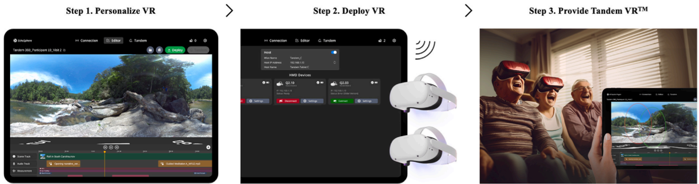
Fig. 2. EchoSphere consists of a tablet and software system to deploy Tandem VR™ to multiple HMDs for synchronized viewing.
