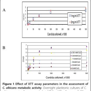
**C.** *albicans* **metabolic activity**. Overnight planktonic cultures of C. *albicans* yeast cells were seeded at  $10^3-5 \times 10^5$  cells per well (30 mm<sup>2</sup> well surface area) and XTT assay was performed as described. (A) Relationship between OD450 and *Candida* cell density at two different XTT concentrations. (B) Effect of CoQ concentration on the linearity range. A representative of three independent experiments is shown.
