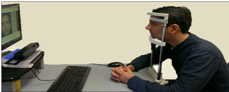
Figure 5. Our ET setup: viewing the subject's face seated on a chin rest, and the near-infrared ET device aiming at the subject's eyes as he observes the monitor. The ET detects movements of less than half a degree of visual angle.
