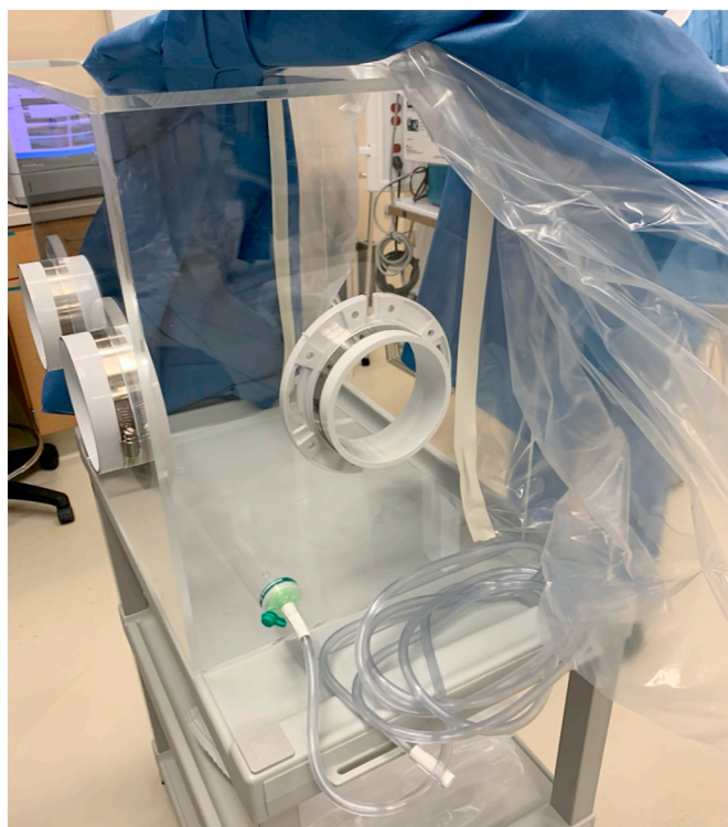
Fig. 1. Rapid prototype of an improved aerosol box.
