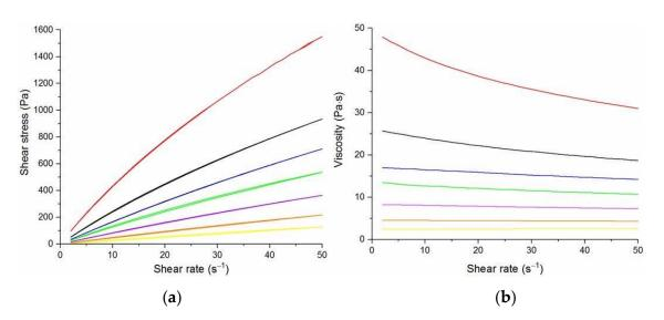
**Figure 5.** Flow curves (**a**) and viscosity curves; (**b**) of solutions of PLDL: **—** 3DMF/1DCM, **—**2DMF/1DCM, **—** PLDL/DMF, **—** 1.5DMF/1DCM, **—** 3DMF/1Acetone, **—** 2DMF/1Acetone, **—** 1.5DMF/1Acetone.
