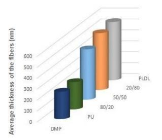
Figure 13. Thickness of the fibers electrospun from DMF cotton liquids without dilution.
