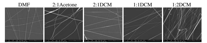
**Figure 7.** SEM images of electrospun fibers of PU/PLDL 80/20. Needle diameter: DMF—0.8 mm; 2:1Acetone, 2:1DCM—0.45 mm, 1:1DCM, 1:2DCM—0.6 mm.
