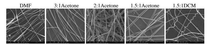
Figure 10. SEM images of electrospun fibers of PLDL. Needle diameter 0.6 mm.
