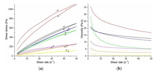
**Figure 4.** Flow curves (**a**) and viscosity curves; (**b**) of solutions of 20/80 PU/PLDL: **—** 2DMF/1DCM, **—** 1.4DMF/1DCM, **—** 20/80/DMF, **—** 1.1DMF/DCM, **—** 1.44DMF/1Acetone, **—** 2DMF/1Acetone, **—** 1.1DMF/1Acetone.
