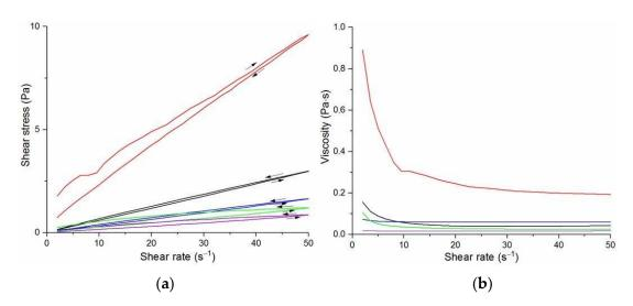
**Figure 3.** Flow curves (**a**) and viscosity curves; (**b**) of solutions of 50/50 PU/PLDL: **-** 50/50/DMF, **-**2DMF/1DCM, **-**2DMF/1Acetone, **-**1DMF/2DCM.
