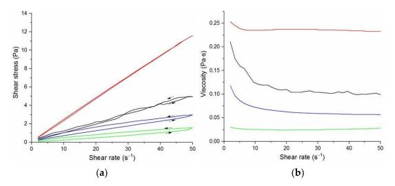
**Figure 2.** Flow curves (**a**) and viscosity curves; (**b**) of solutions of 80/20 PU/PLDL: **-** 80/20/DMF, **-** 2DMF/1Acetone, **-** 1DMF/1Acetone, **-** 1DMF/2Acetone.
