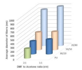
Figure 11. Thickness of the fibers electrospun from cotton liquids diluted with acetone.
