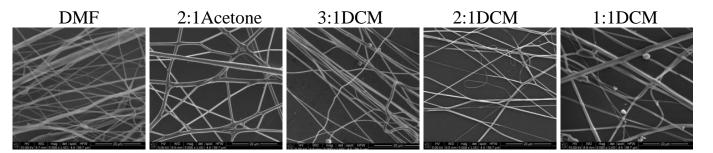
**Figure 8.** SEM images of electrospun fibers of PU/PLDL 50/50. Needle diameter: DMF, 2:1Aetone, 3:1DCM, 2:1DCM—0.6 mm; 1:1DCM—0.8 mm.
