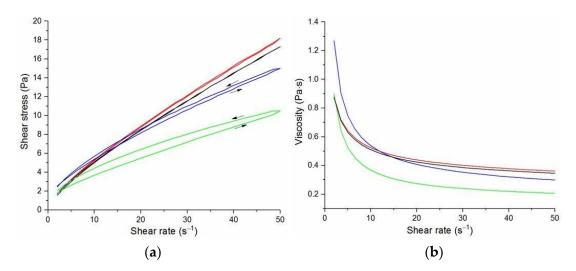
**Figure 1.** Flow curves (**a**) and viscosity curves; (**b**) of solutions of PU: - PU/DMF, -2DMF/1Acetone, -2DMF/1DCM, -1DMF/1DCM.
