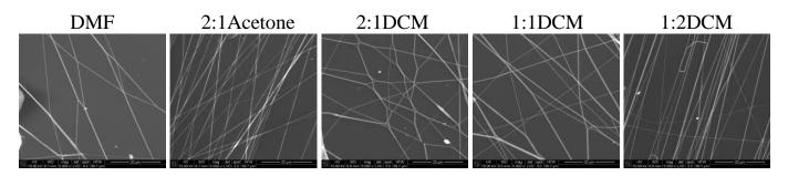
**Figure 6.** SEM images of electrospun fibers of polyurethane. Needle diameter: DMF, 2:1Acetone, 2:1DCM, 1:1DCM—0.6 mm; 1:2DCM—0.45 mm.
