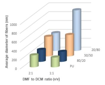
Figure 12. Thickness of the fibers electrospun from cotton liquids diluted with dichloromethane.
