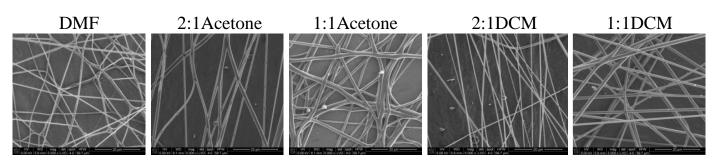
Figure 9. SEM images of electrospun fibers of PU/PLDL 20/80. Needle diameter 0.6 mm.
