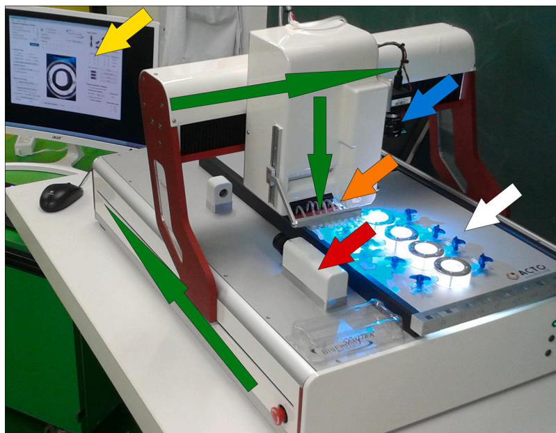
Fig. 1. BioSpotter (BioFluidix, Freiburg, Germany): 3 axis of application are indicated as directions (green arrows); the high resolution camera for documentation, cornea recognition and mapping (blue arrow); stroboscopic camera for volume calibration (red arrow); working surface (white arrow); integrated computer system for control (yellow arrow); dispensing mechanism (orange arrow). (For interpretation of the references to colour in this Figure legend, the reader is referred to the web version of this article).
