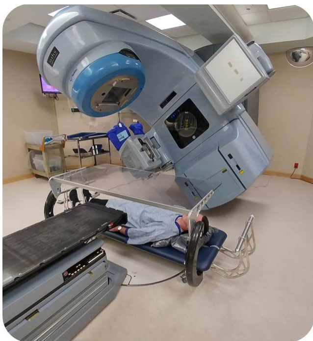
FIG. 4. Photo of the treatment bed, in position for treatment with patient laying supine. Treatment beam is directed toward patient head.
