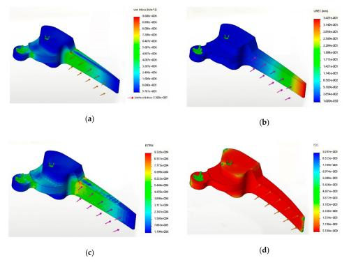
**Figure 4.** Graphical output obtained after assaying a component made of a 50 wt % CF-reinforced composite under 20 N loads: (a) Von Mises; (b) Net displacements; (c) Strain; (d) Safety factor.
