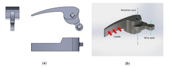
**Figure 3.** Digital mockup of the car interior door handle used as our test case: (a) Normalized views; (b) Perspective view.
