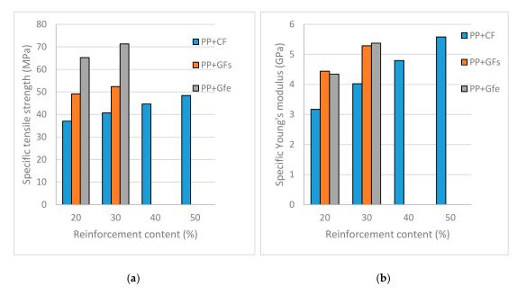
**Figure 2.** Specific tensile properties of curauá, and uncoupled and coupled glass fiber-reinforced polypropylene composites: (a) Specific tensile strength; (b) Specific Young's modulus.
