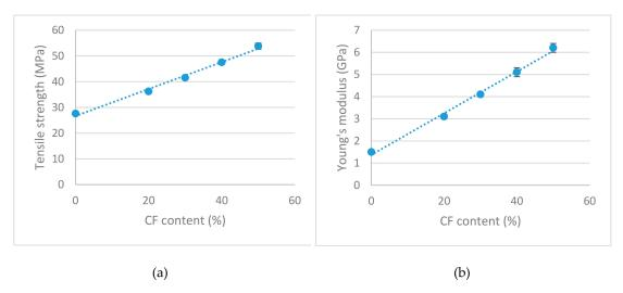
**Figure 1.** Evolution of the tensile properties of the composites against reinforcement contents: (a) Tensile strength; (b) Young's modulus.
