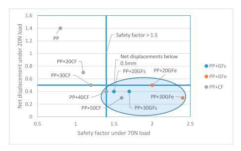
**Figure 5.** Combined requirements for the normal use and misuse conditions. The ellipse encircles the suitable materials that fulfill both requirements.
