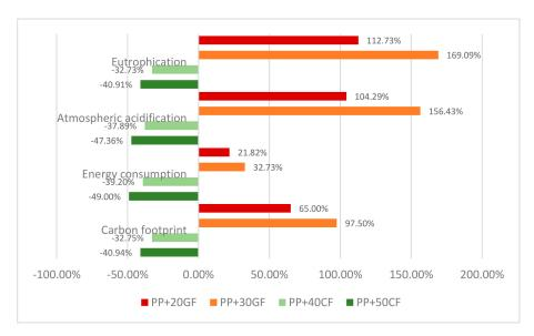
**Figure 6.** Percentage differences between the environmental impact of a polypropylene (PP) component and curauá mechanical pulp (CF)- and glass fiber (GF)-based composites.
