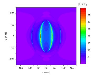
**Figure 10.** Electric field map of a single nanopocket. Electric field enhancement  $|E/E_0|$  with respect to the incident electric field  $E_0$  at the top surface of the nanopocket. The polarization direction is along the short ellipse axis.
