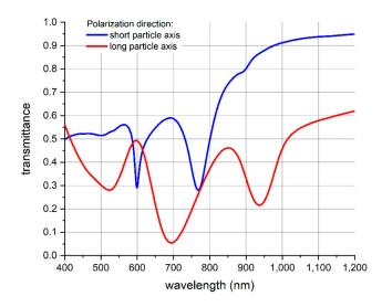
**Figure 9.** Optical simulation results of the transmittance spectrum of the nanopocket array on a glass substrate. The transmittance is plotted in dependence of the polarization direction of the incident light beam. The blue line shows the transmittance for incident light polarized along the short ellipse axis and the red line shows the transmittance for polarization along the long ellipse axis.
