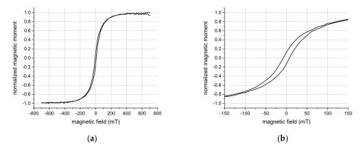
**Figure 13.** Vibrating sample magnetometer (VSM) measurements of the fabricated three-material multifunctional nanopockets: (**a**) obtained hysteresis loop with magnetic field strengths that saturate the magnetic moment of the nanopockets; (**b**) zoom into the hysteresis loop.
