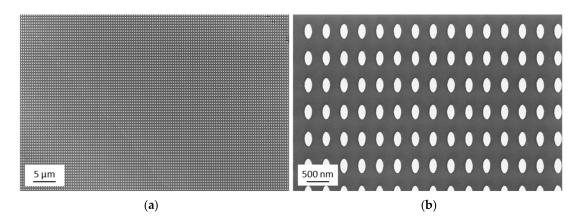
**Figure 2.** Final ultraviolet nanoimprint lithography (UV-NIL)-structured surface. Scanning electron microscope (SEM) after the imprint and the etching processes: (**a**) overview SEM image; (**b**) detailed SEM image.
