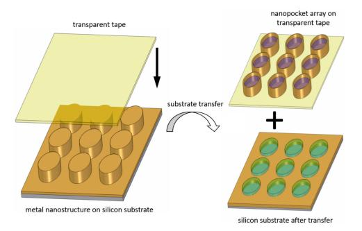
**Figure 4.** Schematic sketch of the substrate transfer from solid silicon to a transparent substrate. On removal of the transparent substrate, nanopockets are created. While the imprint resist stays inside the nanopockets, the lift-off resist remains on the original substrate.
