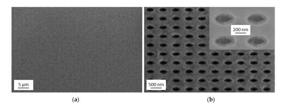
**Figure 6.** SEM imaging of the substrate after the tape transfer step: (**a**) overview SEM image; (**b**) detailed SEM image and a high magnification image of four of the transferred pillars in the insert on the top right.
