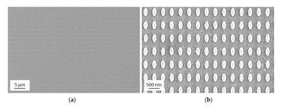
**Figure 3.** Nanostructure array after the sputter process resulting in a Au layer of 50 nm thickness: (a) overview SEM image; (b) detailed SEM image.
