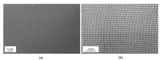
**Figure 5.** SEM imaging of the opening-up nanopocket array on the polyimide tape after depositing a 20 nm thick Au layer on top of the structure for sample preparation: (**a**) overview SEM image; (**b**) detailed SEM image.
