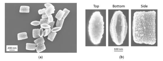
**Figure 12.** SEM images of the fabricated three-material multifunctional nanopockets: (**a**) overview SEM image of randomly oriented nanopockets; (**b**) detailed SEM image with higher magnification of the top, bottom and side view of a nanopocket.
