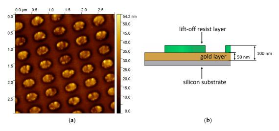
**Figure 7.** Scanning force microscopy (SFM) image of the substrate after the tape transfer process and schematic sketch of the layer thicknesses. (**a**) The remaining elliptical pillars can be observed by SFM imaging. The height of the imaged structure is indicated by the color bar at the right of the SFM image. (**b**) Schematic sketch of the cross section of the sample indicating the layer thicknesses.
