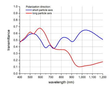
**Figure 8.** Optical transmittance spectrum measurements of the nanopocket array on a transparent film. The transmittance was measured in dependence of the polarization direction of the linearly polarized incident light beam. Polarization of the incident light parallel to the short ellipse axis corresponds to the blue line, while the red line is the measured transmittance for the case of polarization aligned parallel to the long ellipse axis.
