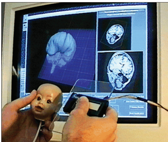
Figure 1: A user selected a cutting plane of a mannequin head with the props interface showing the corresponding MRI image cuts part of preoperative surgical planning. [38] Permission for use obtained by IOS Press BV
