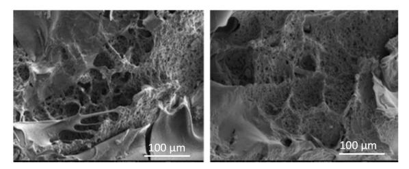
Figure 3. SEM micrographs of p(HEMA-co-AGE) cryogels.
