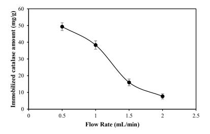
**Figure 5.** Effect of flow rate on catalase binding capacity of p(HEMA-co-AGE) cryogel [catalase concentration: 1.0 mg/mL in 50 mM pH 6.0 phosphate buffer; T: 25 °C].
