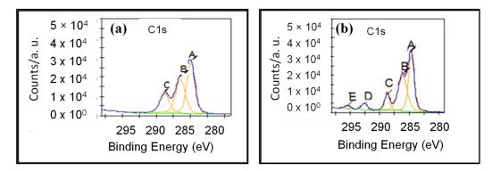
Figure 4. (a) C(1s) XPS Spectra of p(HEMA) and (b) p(HEMA-co-AGE) cryogels.
