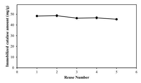
**Figure 8.** Reusability of p(HEMA-co-AGE) cryogel [flow rate: 1.0 mL/min; catalase concentration: 1.0 mg/mL; T: 25 °C].
