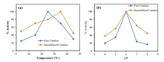
**Figure 7.** (a) Effects of temperature on % activity of free catalase and immobilized catalase enzymes onto p(HEMA-co-AGE) cryogels [reaction conditions: 50 mM phosphate buffer, pH 6.0], and (b) effects of pH on % activity of free and immobilized catalase enzymes onto p(HEMA-co-AGE) cryogels [reaction conditions: 50 mM phosphate buffer, T = 35 °C].
