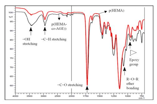
Figure 2. FTIR-ATR spectra of p(HEMA) and p(HEMA-co-AGE) cryogels.
