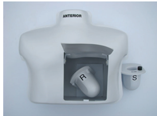
FIGURE 4: The SNMMI 2012 Cardiac SPECT phantom simulator showing the myocardium insert, manufactured by Medical Designs, Inc. (MDI). Figure is obtained from citation [16].
