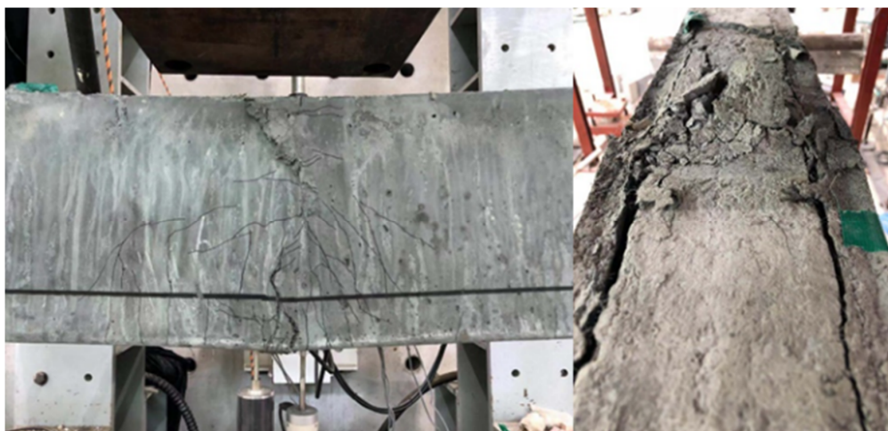
Figure 10. Compressive failure (B-3J).
