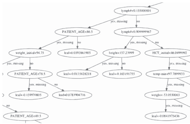
Figure 4 Representative portion of a single tree from the XGBoost model. The final model contains 100 unique trees which combine to yield the model prediction. Terminal node (“leaf”) values represent the log odds of the probability of intubation. To arrive at the predicted probability, the values of the appropriate leaves of each tree in the model are summed and transformed into a probability using the logistic function. XGBoost, eXtreme Gradient Boosting; HCT, hematocrit.
