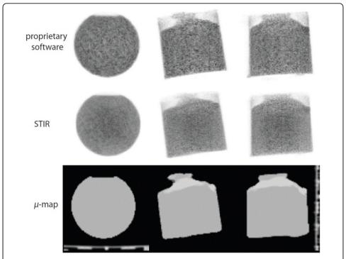
**Figure 1** Image reconstruction of the phantom using Siemens proprietary software (top) and STIR (middle). Bottom: the MRI derived  $\mu$ -map.
