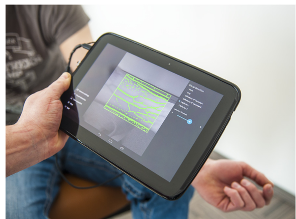
Figure 3 Prototype during the suitability assessment (pre-screening). An example of sufficient visibility of the subcutaneous veins on the inner elbow with additional visualization of the vein pattern using the Laplacian I processing.
