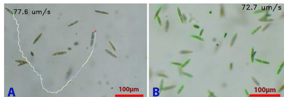
Figure 14. Microalgae tracking. (A) Tracking a E. gracilis cell to determine its trajectory. Cell concentration in the well was 2 \times 10^5 cells \text{mL}^{-1} . The tracking is performed with a OpenCV script allowing the user to click on the cell to track. The cell’s path will then be drawn in real time on the live video. (B) Analysis of the direction of movement of all the cells in a culture. Green lines allow determining the direction and speed of the algae (the length of the lines is relative to the speed). Both scripts allow obtaining the speed in \mu\text{m}/\text{s} .
