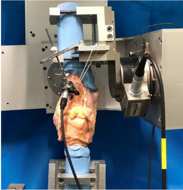
**Figure 1.** Robotic testing system with a right knee. The manipulator, which worked with the universal force-torque sensor, was placed on the end-effector. The tibia was fixed on the end-effector, and the femur was fixed to the lower part of the device using metal clamps. An adjustable tension rod was attached to the plate, which was connected to the tibial clamp, and the force gauge was attached to the tendon graft.
