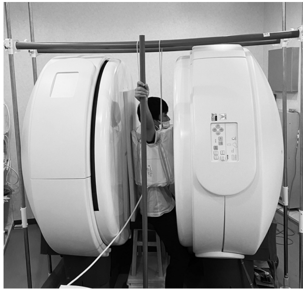
Fig. 3. Image of gravity magnetic resonance imaging apparatus. The quadrature body coil was suspended above the seated participant by a wire and the height was adjusted to include the entire scapula in the measurements.
