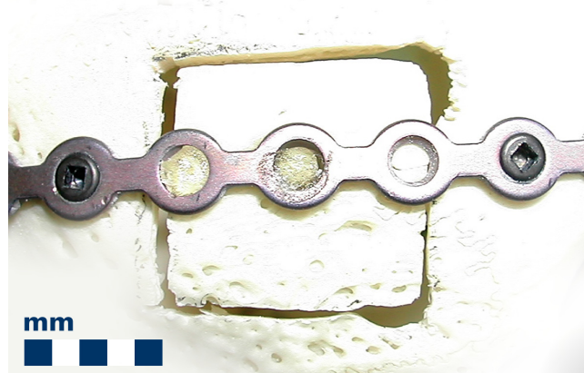
Figure 2 Partially adhesive fixation of an osteosynthesis plate. The new technique for the adhesive fixation of an osteosynthesis plate. The osteosynthesis plate is fixed on a rabbit bone sample with a square-cut damage of ca. 1 cm 2 . On sufficient cortical bone mass structures the plate is fixed with screws as usual. On the fragile bone fragment the plate is adhesively fixed to the bone of the square-cut damage with a PMMA bone cement and with an amphiphilic bone bonding agent as an intermediate layer.
