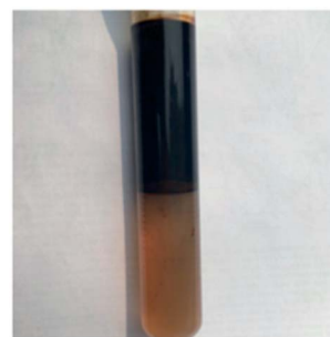
Fig. 6 Photograph of crude-oil-in-simulated formation water middle phase microemulsion taken after 3 weeks of settling 45^\circ\text{C} .
