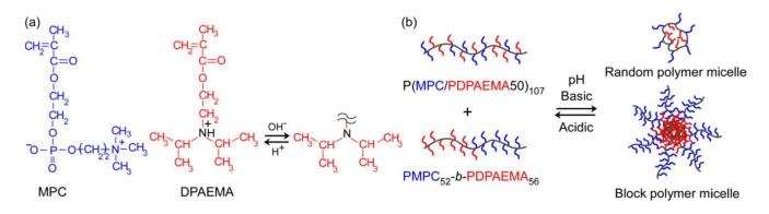
**Figure 1.** (a) Chemical structures of MPC and DPAEMA, and pH-responsive behavior of DPAEMA. (b) Conceptual illustration of the pH-induced formation of separated micelles in a mixed aqueous solution of the random and block copolymers consisting of MPC and DPAEMA.
