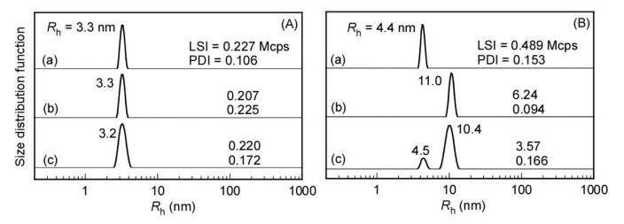
**Figure 4.** Hydrodynamic radius ( $R_h$ ) distributions of (**a**) P(MPC/DPAEMA50)<sub>107</sub>, (**b**) PMPC<sub>52</sub>-*b*-PDPAEMA<sub>56</sub>, and (**c**) an equimolar mixture of the random and block copolymers at a total polymer concentration of 10 g/L in 0.1 M NaCl at pH 3 (**A**) and 10 (**B**) at 25 °C.
