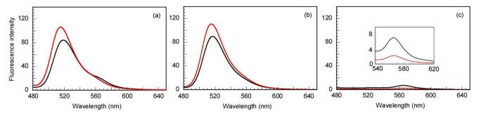
**Figure 7.** Fluorescence spectra of A488-labeled block and A555-labeled random copolymers (**a**), A488-labeled block copolymer (**b**), and A555-labeled random copolymer (**c**) in mixtures with nonlabeled random and block copolymers at a total polymer concentration of 10.0 g/L in water at pH 2 (black) and 11 (red).  $\lambda$ ex = 450 nm, the excitation and emission slit widths were 20 and 2.5 nm, respectively. A488 = Alexa Fluor 488 C5 maleimide; A555 = Alexa Fluor 555 C2 maleimide.
