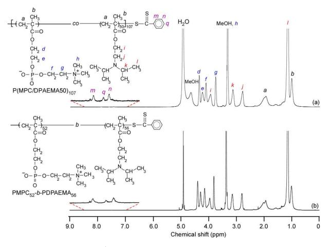
**Figure 2.** <sup>1</sup>H NMR spectra of (**a**)  $P(MPC/DPAEMA50)_{107}$  and (**b**)  $PMPC_{52}$ -*b*-PDPAEMA<sub>56</sub> in methanol- $d_4$  at 25 °C.
