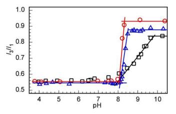
**Figure 3.** Fluorescence peak intensity ratio  $(I_3/I_1)$  of pyrene in the presence of (MPC/DPAEMA50)<sub>107</sub> ( $\Box$ ), PMPC<sub>52</sub>-*b*-PDPAEMA<sub>56</sub> (o), and their equimolar mixture ( $\Delta$ ) in 0.1 M NaCl at a total polymer concentration of 1.0 g/L as a function of the solution pH.
