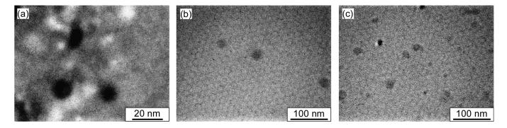
**Figure 5.** Representative transmission electron microscopy (TEM) images of (**a**)  $P(MPC/DPAEMA50)_{107}$ , (**b**)  $PMPC_{52}$ -*b*-PDPAEMA<sub>56</sub>, and (**c**) an equimolar mixture of the random and block copolymers at a total polymer concentration of 10 g/L in 0.1 M NaCl at pH 10.
