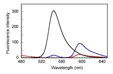
**Figure 8.** Fluorescence spectra of A488-labeled block polymer (black), A555-labeled random polymer (red), and their equimolar mixture (blue) in acidified dimethylsulfoxide;  $\lambda ex = 450$  nm, the excitation and emission slit widths were 20 and 1.0 nm, respectively. A488 = Alexa Fluor 488 C5 maleimide; A555 = Alexa Fluor 555 C2 maleimide.
